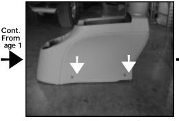
**STEP 8:** Remove the four screws (two per side) from the sides of the console.
